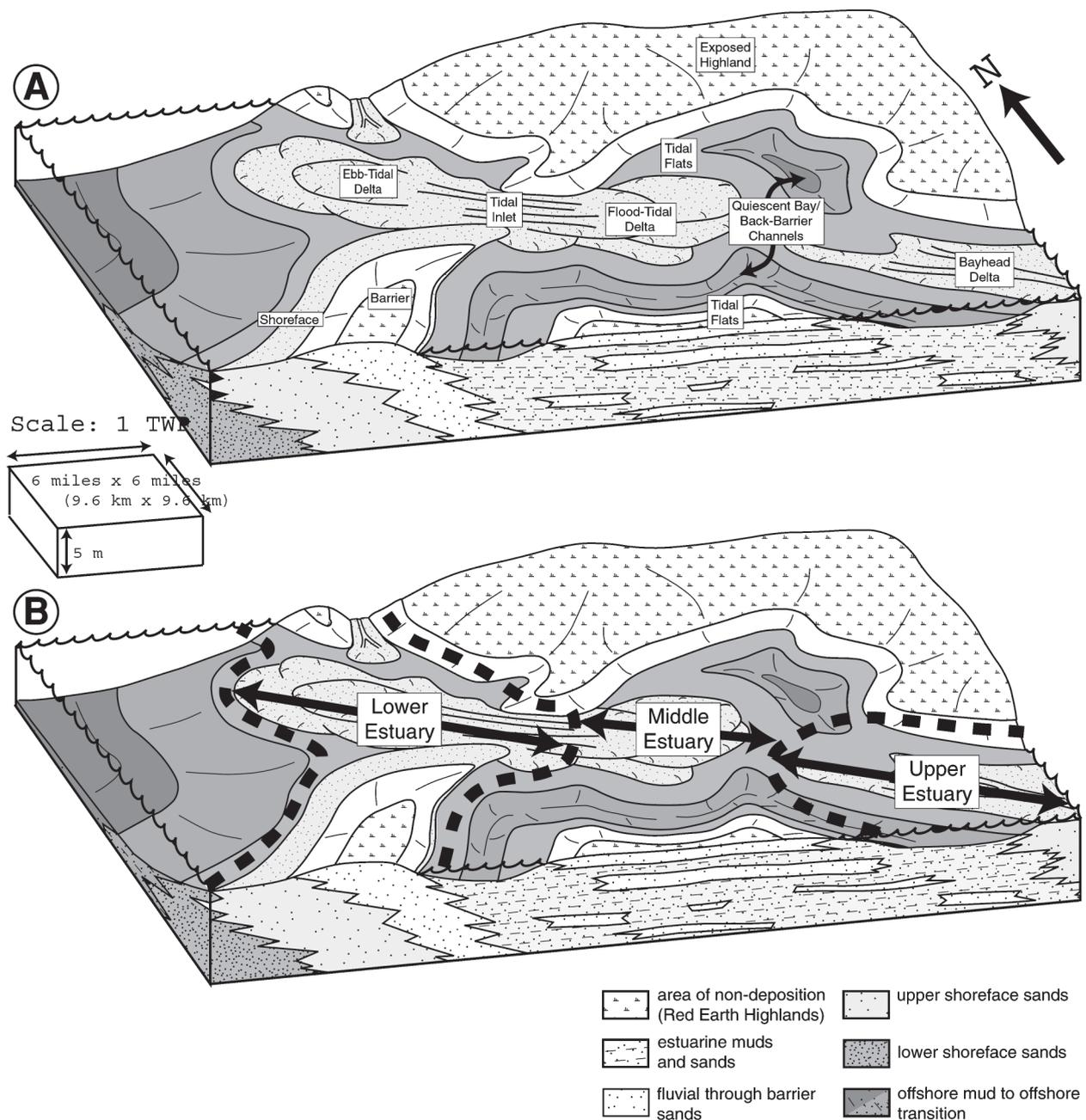
Fig. 3. A: The wave-dominated estuary facies model interpreted for the Bluesky Formation in the Cadotte study area (modified from Hubbard *et al.* 2002). B: Estuarine divisions (upper, middle and lower) as defined in this study.
