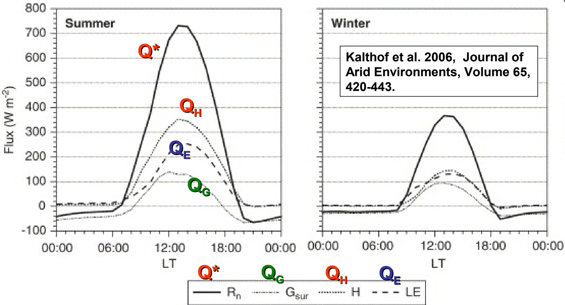
Mean daily cycle of the energy balance components (net radiation,  $R_n$ ; sensible heat flux  $H$ ; latent heat flux  $LE$ ; and soil heat flux,  $G_{sur}$ ) for the summer and winter seasons, averaged over the years 2000–2002 for an arid valley in Chile. Latent heat flux less important than previous example.
