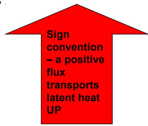
Upward flow of latent heat on average,  $Q_E > 0$
