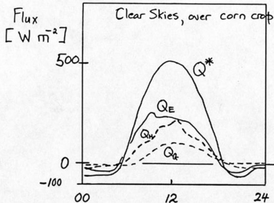
example of the daily cycle; this case, surplus daytime radiant energy shared about equally by latent and sensible heat fluxes to the air
