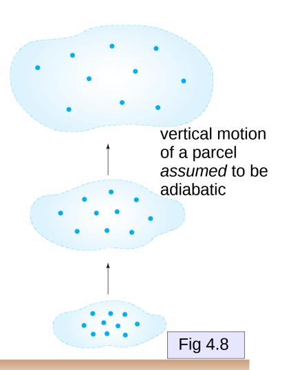
If a parcel at the surface (z=700 m) has  $T=13^{\circ}\text{C}$  and it is lifted adiabatically, what is its temperature at z=1000 m?
