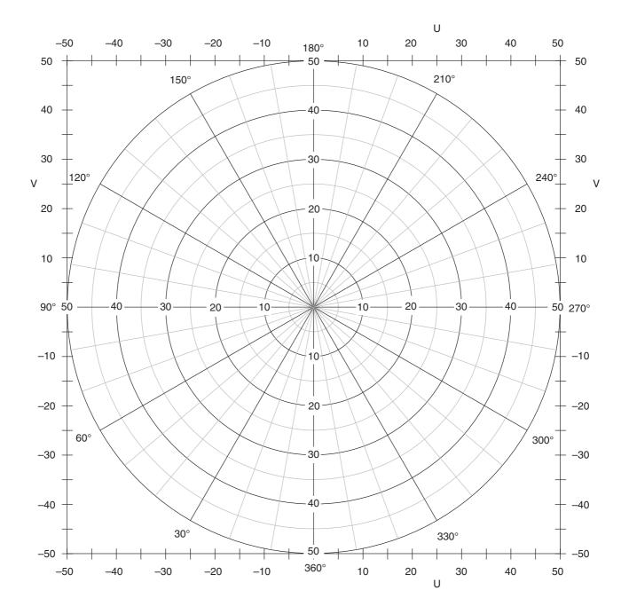
**Figure 16.51** Blank hodograph for you to copy and use. Compass angles are direction winds are <u>from</u>. Speed-circle labels can be changed for different units or larger values, if needed.
