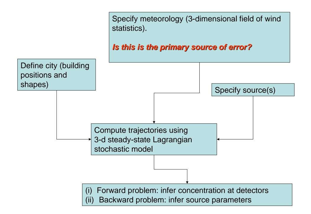
Using a Lagrangian stochastic model to compute the concentration field due to a gas source in urban winds
