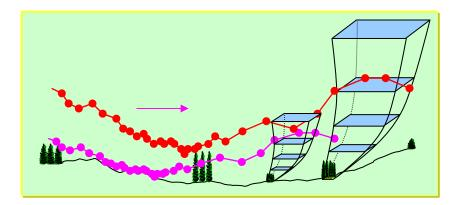
Thomson's well-mixed LS model for 2-D Gaussian, vertically-inhomogeneous turbulence
