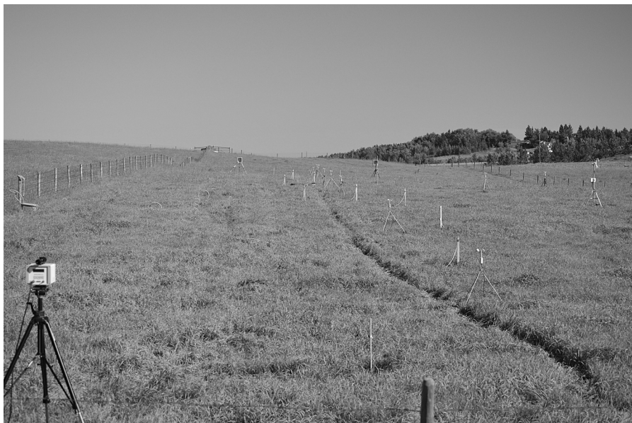
Fig. 1. A view of “plot 22” looking towards the north from the southern boundary fence. The origin of the coordinate system lies at the junction of the two visible fences, just out of sight at the lower left of the photograph. The light path of the laser gas detector at lower left runs northward, parallel to the fence defining the western boundary of plot 22, to a reflector seen just below the skyline. Also visible: cup anemometers, elevated gas release points, and a sonic anemometer at the right of the photo. The distance along the western fence from the origin to the gate on the skyline is 290 m.
