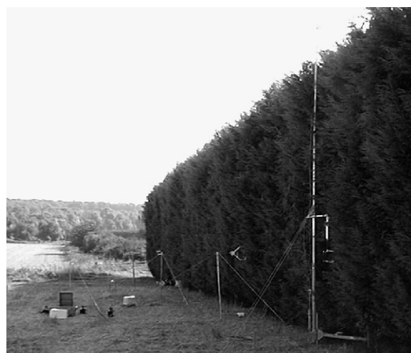
Fig. 2. Eastern side of the cypress hedge “A” (height H = 8 m, thickness X = 3 m) looking (roughly) south towards the access break in the willows (“D”, not visible). A CSAT3 and a Gill sonic anemometer are visible, placed against the face of the hedge.
